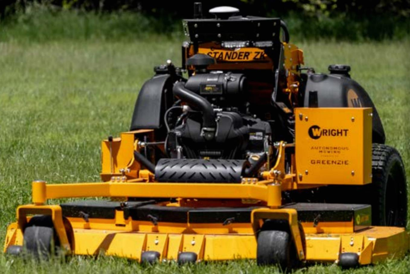
The **AUTONOMOUS ZK** increases your profit by doing more in less time. Easy to use—record the perimeter pass and let the mower cut the middle autonomously and then save that job and stripe angle as a favorite in the app for next week. Seamlessly switch between manual use and autonomous mowing means complete versatility for any job you encounter.
